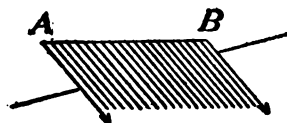
Fig. 2.—Moving line, A B , generates a surface having two dimensions—length and breadth.
